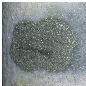
As-bearing pyrite in sandstone
